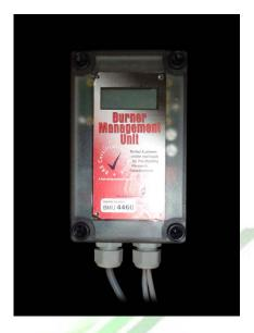
This technology is designed to alter the firing pattern of the boilers to improve their energy efficiency without impairing the performance of the boilers.
